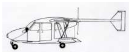
Fig 2 A possible appearance of the aircraft if it had been completed with a Franklin 125hp engine (Del IW). The fairing below the engine is assumed to be similar to that of the Marchetti Riviera which tapers to a point. It cannot end abruptly on the airframe as it does presently. The doors have been drawn based on the locations of three sets of hinge attachment points on the present airframe. The central pillar in the
